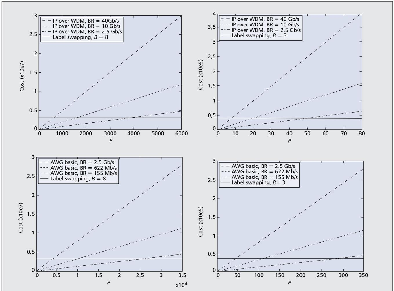
■ **Figure 5.** Cost comparison for different packet switching node architectures and different values of the header bit rate (BR). The nodes have 4 fibers, 32 wavelengths/fiber, 8-bit label length for label swapping, and 3-bit label length for label stripping.
